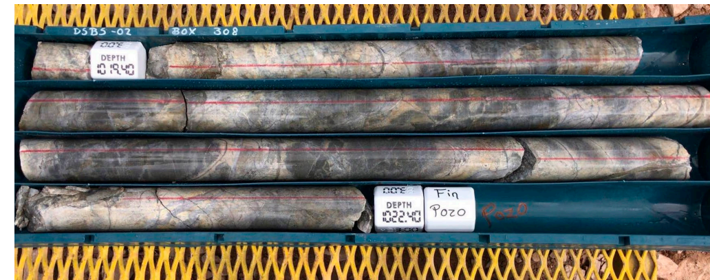
The longest HQ diamond drill hole completed in Bolivia at 1,022.4m at Iska Iska silver-tin polymetallic project. (Source: Eloro Resources)
