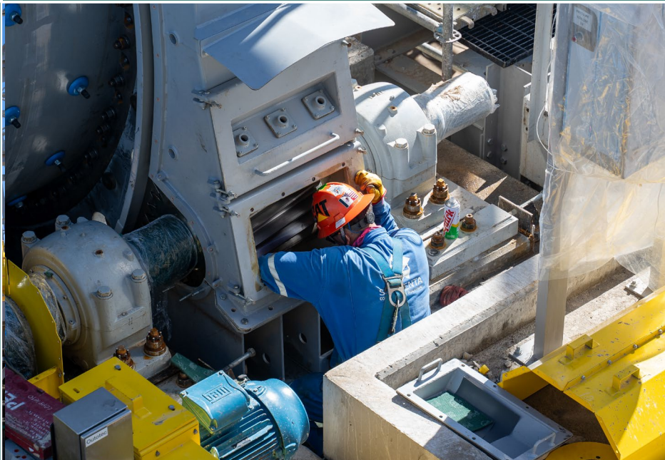
Installation of the pinion gear on the ball mill
