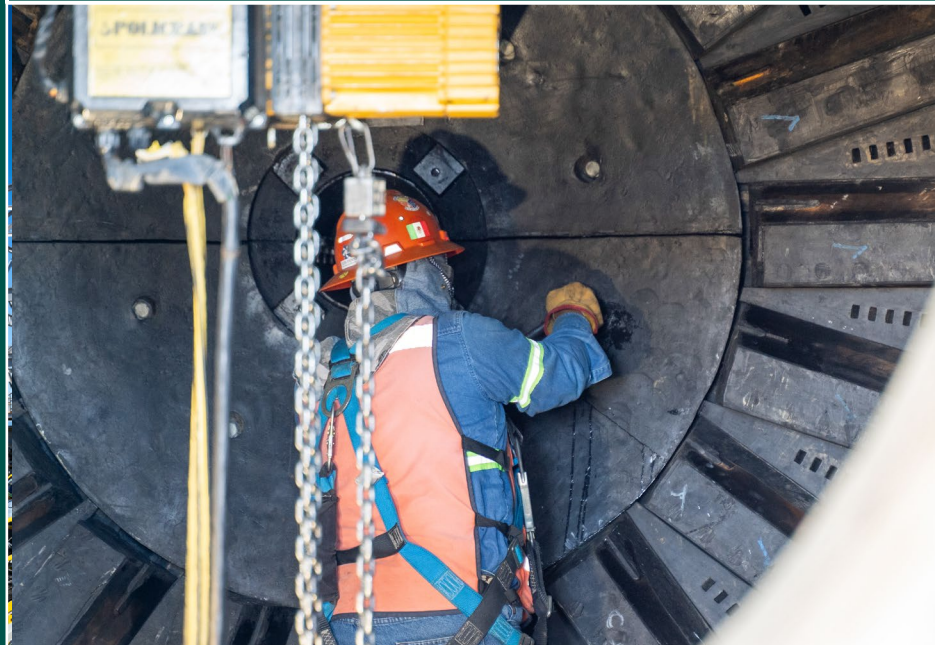
SAG mill liner installation
